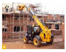
It's not only JCB's revolutionary HiViz range that places the JCB Loadall as one of the safest telehandlers on the market; Our patented load control system and sway frames allows for a safer and more stable load placement, whilst hose burst check valves protect the driver and bystanders in the event of hose failure.
