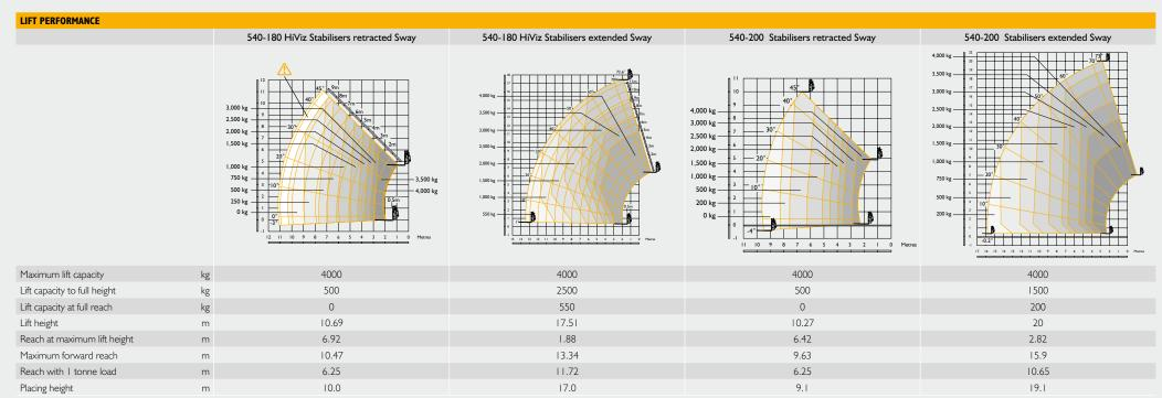
Complies with stability test EN 1459 Annex B. Chassis Levelling (Sway) with stabilisers retracted (Sway angle  $\pm$ 9°).
