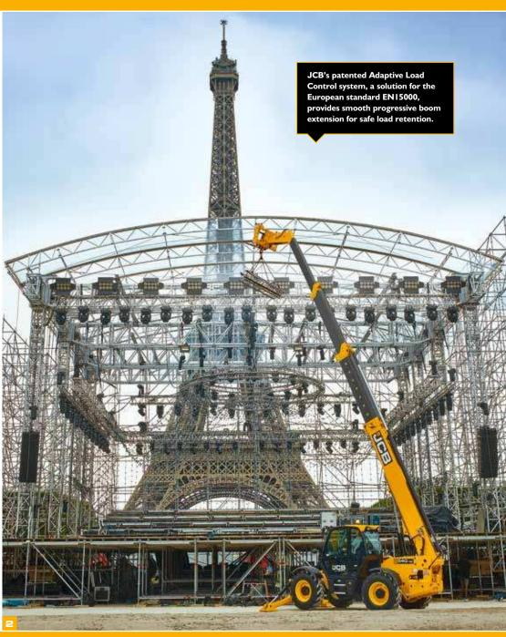
With a 10% reduced turning circle than the 540-170 as well as 1000kg lighter thanks to a shortened chassis and lightweight boom sections, the 540-180 HiViz is one of the most manoeuvrable machines around.
