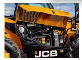
By producing high levels of power and torque even at engine speeds as low as 1300– 1400rpm, the EcoMAX engine can provide fuel-efficient matching of transmission and hydraulics.
