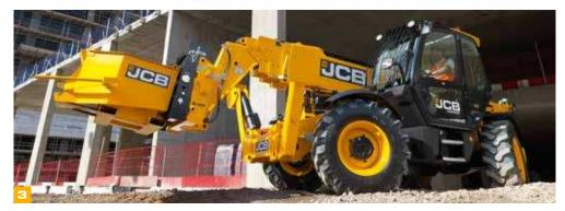
The JCB EcoMAX engine produces its power and torque at low engine speeds, which makes it highly responsive to operate. With a variable geometry turbo for superb performance at low revs, you can expect greater fuel efficiency.\*
