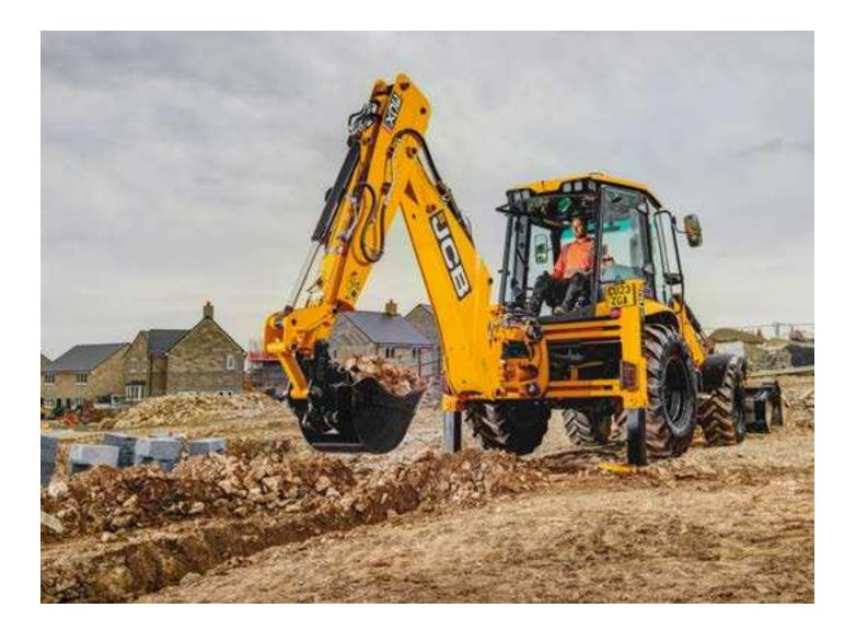
Innovative DUALDRIVE controls enable machine repositioning when using the excavator, without turning the seat. Powerslide hydraulically re-positions the excavator.
